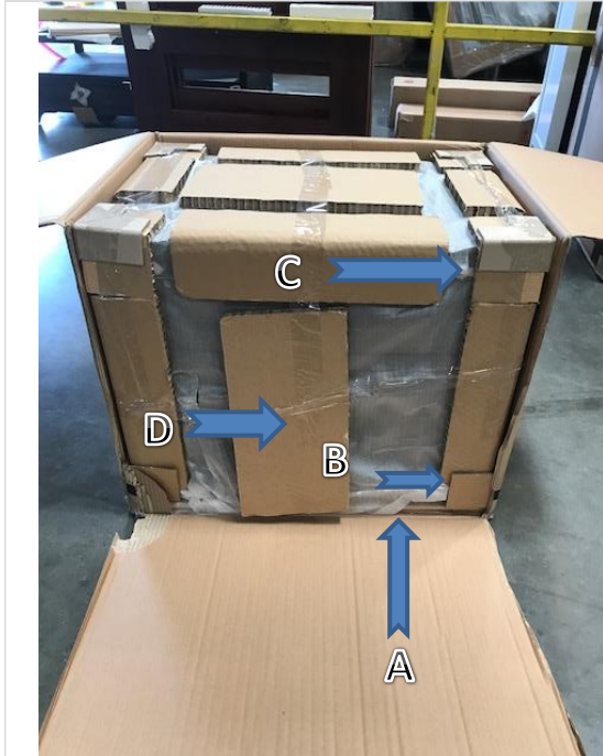
A-Wood pallet protection on floor side B- Leg protection C-Built out corrugate protection on all corners D-Airspace must be filled with foam and cardboard
