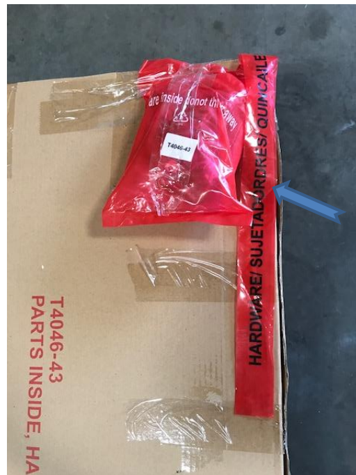
Hardware and loose parts need to be easily identifiable with red ribbon or marked as hardware on carton
